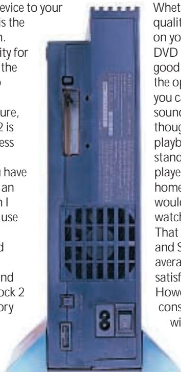
There's optical out for DVD and a hard-disk interface in the UK model
